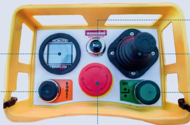
Battery level indicator and operating hours counter
